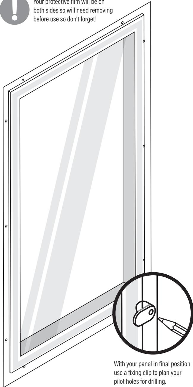
With your panel in final position use a fixing clip to plan your pilot holes for drilling.
