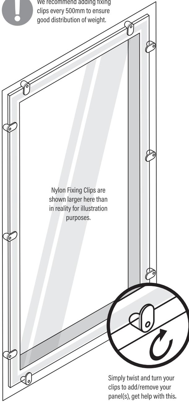
Nylon Fixing Clips are shown larger here than in reality for illustration purposes.
